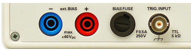
Location of the BIAS FUSE at the rear panel
